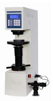
iqualitrol SHB-3000D adopts the motorized test force application without weights, and uses 0.5% accuracy compression sensor to feedback and the CPU control system to automatically compensate the test force lost during the testing.
